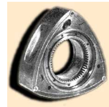
Piston of a Wankel rotary engine (exceptional case)
