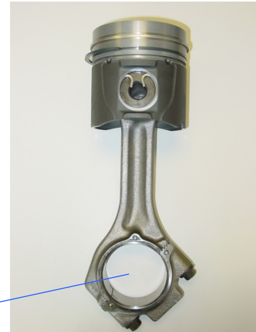
Assembly Piston – Ring – Connecting rod
